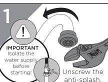
Remove the anti-splash and filter from housing.
